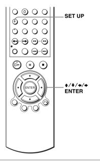
Press SET UP when the DVD player is in stop SET UP mode, then press 4/4 to select (OPTION), then press ENTER.
